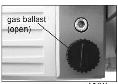
For **condensable vapors** (water vapor, solvents, etc.):
